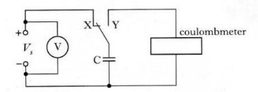
When the switch is in position X, the capacitor charges up to the supply voltage,  $V_s$ . When the switch is in position Y, the coulombmeter indicates the charge stored by the capacitor.
