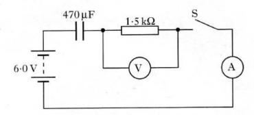
The capacitor is initially uncharged.
