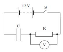
The capacitor is initially uncharged. Switch S is now closed. Which graph shows how the potential difference, V, across R, varies with time, t?
